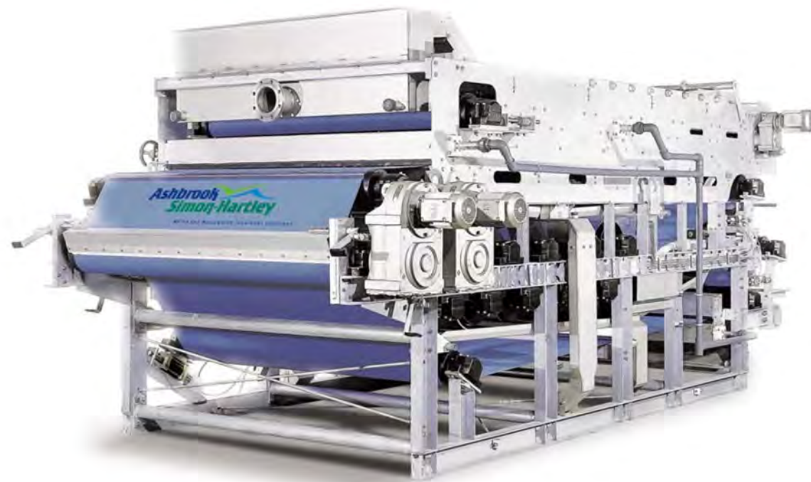
3-Belt BFP Operation (Courtesy of Ashbrook Simon-Hartley)
